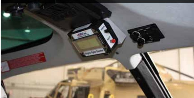
Like AKV's cycle counters, the ETM1000 is simple to install, connects to existing airframe and engine signal generators, is field programmable, and has no associated subscription fees — customers own their own data. "It's a full turn-key system," said Gunn. "I've provided a lot of capability for the price."
